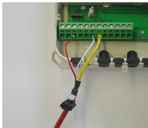
Figure 12: Example of the connection of a shielded cable in two-wire system
