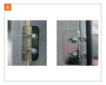
Before finally closing the nuts, check the correct alignment of the lock with the hook / strike plate. Perform repeated opening and closing of the open tailgate lock.
