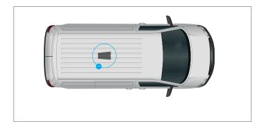
If you have 1 fan, place it as close as possible to the centre point of the roof which can be determined by measuring from the bulkhead to the tailgate or rear doors.
