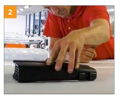
2. Place the foam gasket underneath the Easy Aero and push the tubes through the holes with the grille at the front. *Note:* the foam gasket should be fitted at all times! The foam gasket is available separately in a range of thicknesses: ask our specialists for advice on the correct thickness to use.
