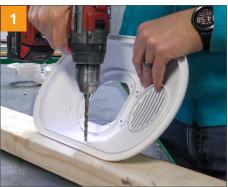
Drill holes in the stipulated places on the inside of the cover plate.
