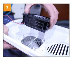
Place the finger protector (grille) and fan in the cover plate correctly (with the arrow pointing upwards).
