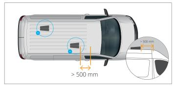
If you have 2 fans, place them diagonally so that they are evenly spaced. Divide the space into 3 equal parts lengthwise (measured from the bulkhead to the tailgate or rear doors) and place the Easy Aero 1/3 from the front and 1/3 from the rear and widthwise halfway along the half-diagonal.
