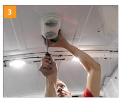
Screw the cover plate onto the inside of the roof using the screws provided. The roof fan is installed: easy!
