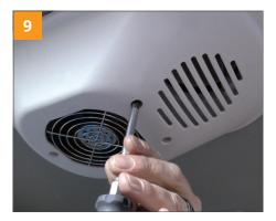
Secure the Easy Aero module cover plate using the three screws provided.
